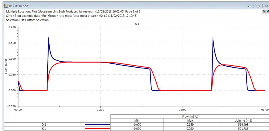
**Figure 8 Forcemain Flow Results, Air Valves Included**
