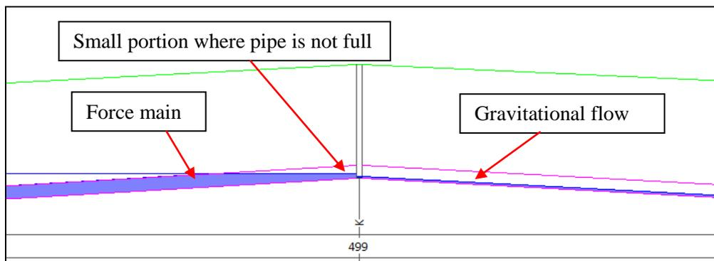
**Figure 3 Top of Rising Main with Pressure Model**
